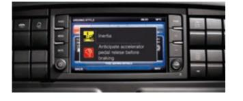
Fuel-saving suggestions appear on screen while the vehicle is running (they taking into account gears, braking, engine braking, acceleration and inertia).
