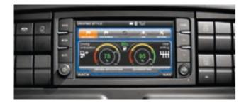
The **DRIVING STYLE EVALUATION** system processes the data acquired from the engine, vehicle and GPS with an advanced algorithm that evaluates fuel saving performance. The score takes into account the difficulty of the mission.
